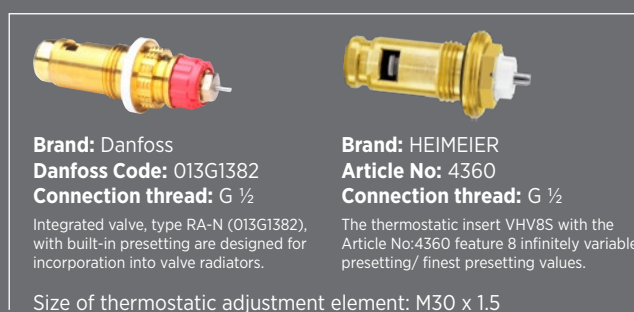
Thermostatic Valve Insert
